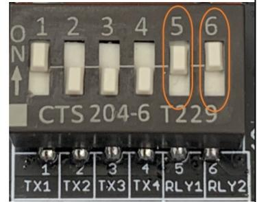
4. On the DIP switch, indicate which transmitter channels will output through Relay 1 and Relay 2 terminals by setting the corresponding DIP. For example, the image to the right shows Tx1 outputting through Relay1, and Tx2,3 and 4 outputting through Relay2.
