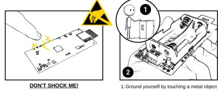
WEL-200T components are sensitive to static shocks (ESD) 2. Hold the circuit board only by the edges
