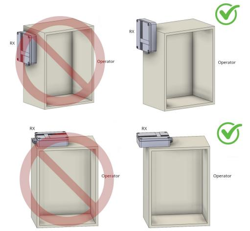
Even though there are 4 mounting holes on the RX, it's OK to just use 2 holes so that the RX will overhang the operator box as shown above. When mounting the RX, make sure the cable grip is facing down or to the side, never up – this will prevent water from getting in.
