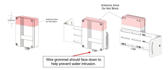
Never install the RX inside an operator box, especially a metal one:
