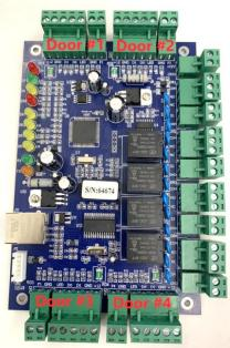
b. At a minimum, the two datalines (**D0 and D1**) and the **GND** terminal need to be connected to the wiegand device. Wire color to these terminals ultimately depends on which wiegand reader you are using.
